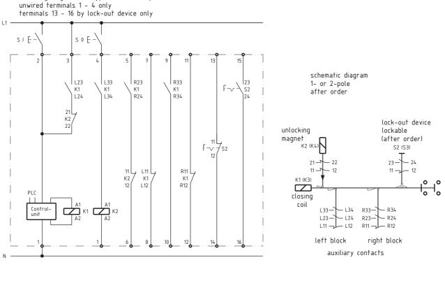
switching diagram for Typ E and ET complete wired unwired terminals 1 – 4 only terminals 13 – 16 by lock-out device only
