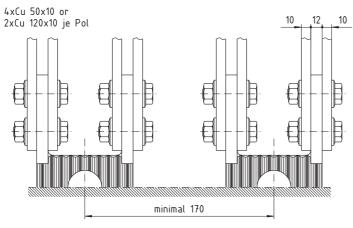
Blade-type parallel or flat-type connections for switch type E...
