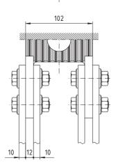
Blade-type parallel or flat-type connections for switch type D....
